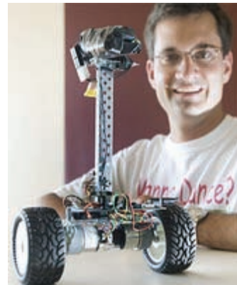
(b) Hanno Sander's balancing robot, initial prototype developed with the Propeller Education Kit and ViewPort software. Photo courtesy of mydancebot.com.
