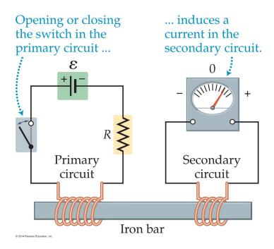
Turning on the current in the left circuit causes a changing magnetic field in the primary coil. The magnetic field propagates through the iron bar and the changing magnetic field causes a current to flow in the secondary circuit.
